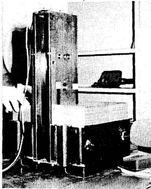
FIG. 4 Lamination stacking tool.
