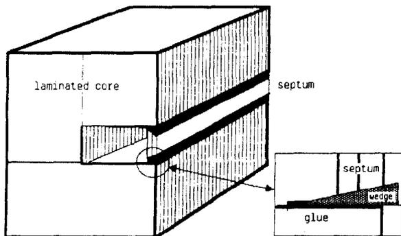
FIG. 2 Glass fibre wedges to retain coil in gap.
