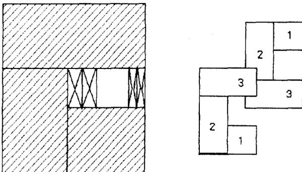
FIG. 3 Magnet lamination construction.
