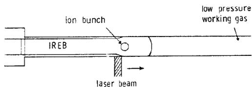
Fig. 1. Ionization Front Accelerator (IFA).
