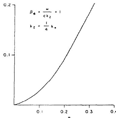
Fig. 3 Locus of Points for which  $v_\phi = c$  in a  $\pi/2$  Structure
