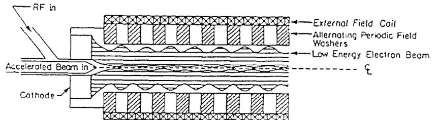
Fig. 1 A Sketch of a Periodic Plasma Waveguide
