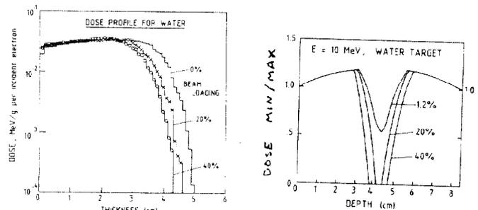
Fig. 7(a) Change in depth dose curves with beam loading. (b) Variation of min/max ratios with beam loading.
