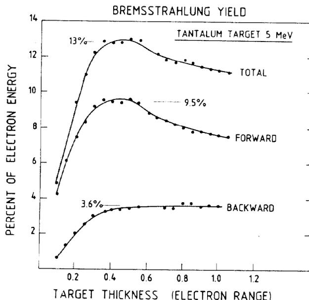
Fig. 2(a) Bremsstrahlung yield vs thickness of radiator.
