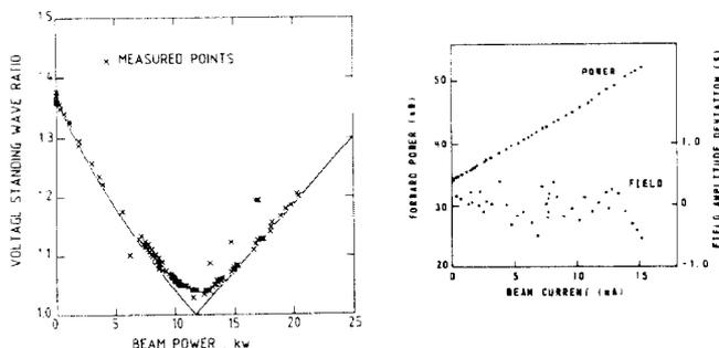
Fig. 8 Effect of beam loading in a cw linac (a) shows the change in impedance match and (b) demonstrates that the fields can be held constant ( $\pm 1\%$ ) at up to 50% loading.
