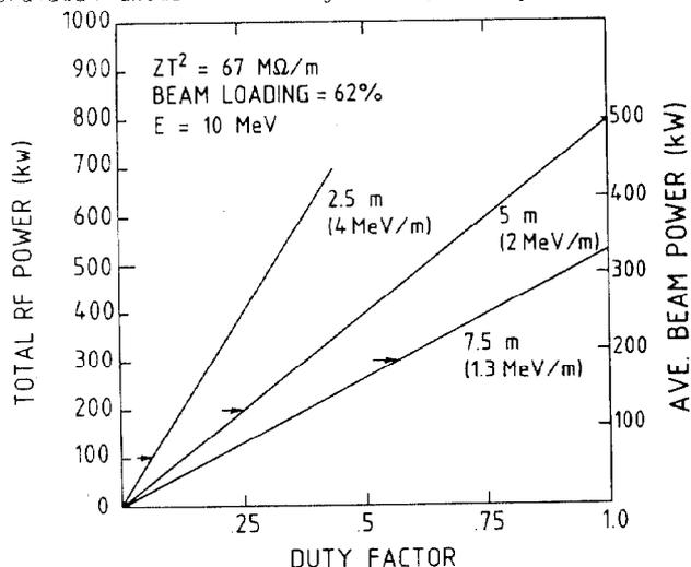
Fig. 9 Design curves for long pulse machine.
