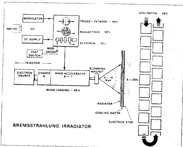
Fig. 5 Component efficiencies for linac irradiator.
