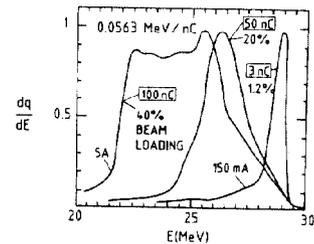
Fig. 6 Typical energy spectra for the LEP injector.
