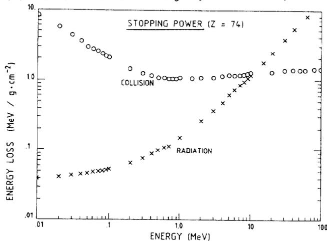
Fig. 1(b) Variation of collision and radiative cross-sections with energy.
