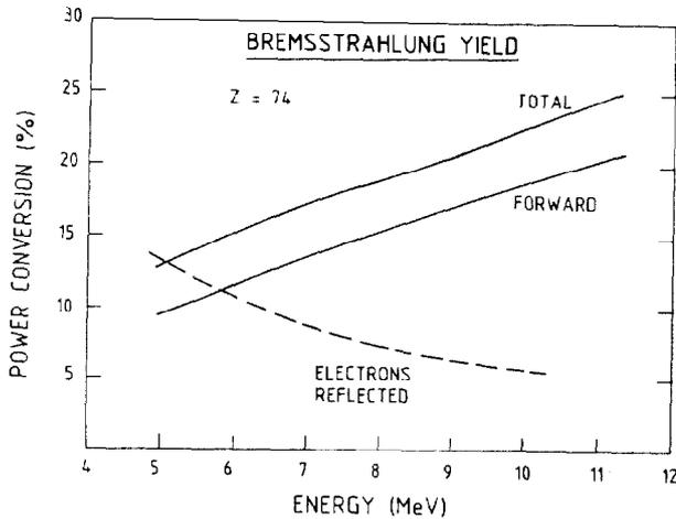
Fig. 2(b) Variation of bremsstrahlung yield with energy.
