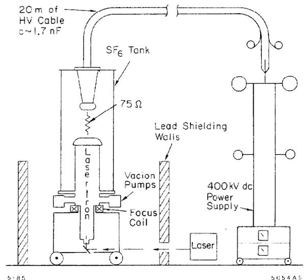
Fig. 5 - Lasertron experimental setup showing the -400 kV dc power supply, laser, lead shielding wall, high voltage cable (and storage capacitor), cable bushing, arc-energy absorbing resistor and the lasertron in its sulfur hexafluoride tank and mounted on a cart.
