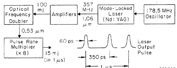
Fig. 6 - Block diagram of the laser which will be modulated at 2856 MHz and will be needed for RF tests of the lasertron.
