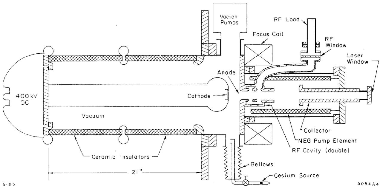
Fig. 4 - Cathode to collector geometry for the lasertron.
