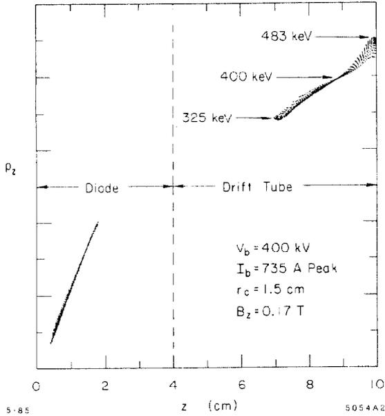
Fig. 2 - MASK computation of longitudinal momentum,  $p_z$ , versus distance from the cathode,  $z$ . The tail of the first pulse is out of the diode accelerating region, thus the energy spread between the front and the back of the bunch is representative of that of the bunched beam before it enters an RF cavity. The normalized fundamental harmonic component of the pulse train,  $I_1/I_0$ , is greater than 1.5.
