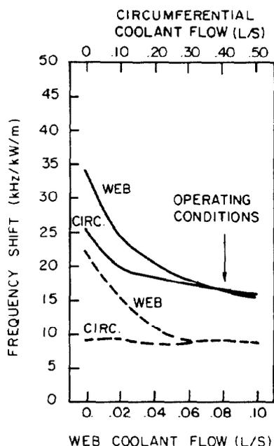
Fig. 3 Calculated frequency shifts (continuous curves) and change in stopband frequency gap (dashed curves) as function of circumferential and web coolant flow rates. Results are shown for fixed web coolant flow of 0.08 L/s (identified by CIRC.) and for fixed circumferential flow rate of 0.43 L/s (identified by WEB).
