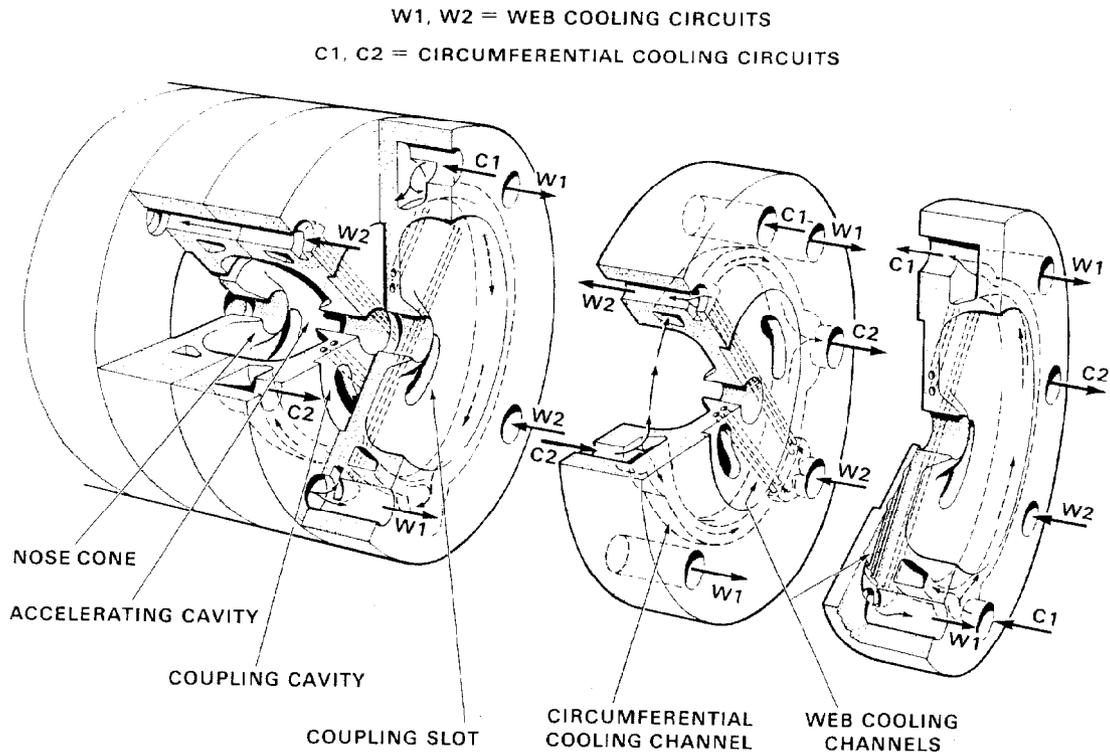
Fig. 2 Cooling channels for the on-axis coupled cavities.
