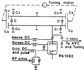
Fig. 6: Schematic diagram of resonant system and final tube.
