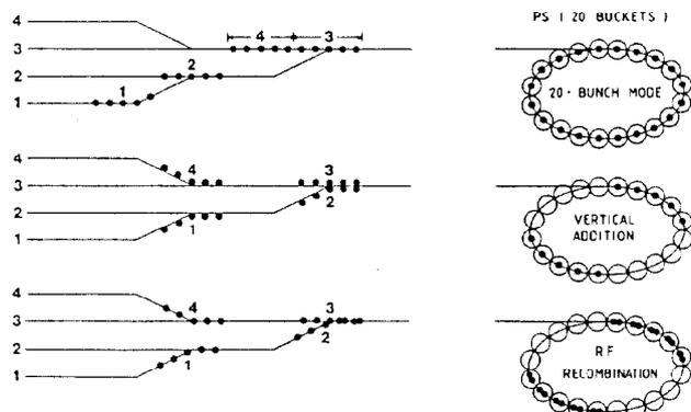
Fig. 2: Schemes for recombining the four PSB rings.
