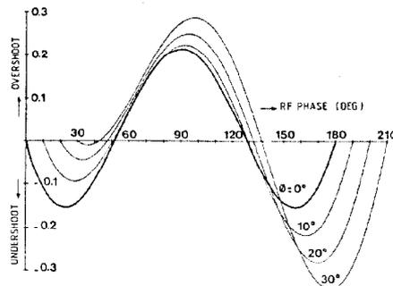
Fig. 7: Weighted relative overshoot along the bunch (φ = phase between sinusoidal deflector and bunch)
