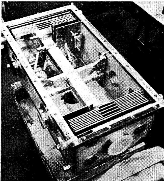
Fig. 5: View of magnet with cover of vacuum tank removed.
