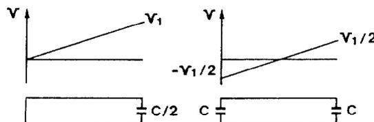
Fig. 3: Voltage distribution for single and double ended arrangements.
