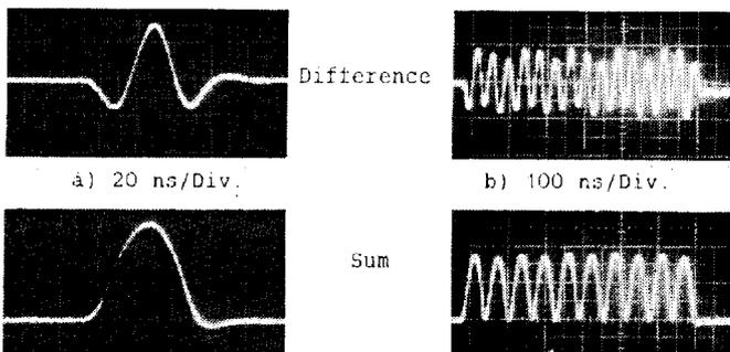
Fig. 9: Sum and difference signals on a position monitor downstream of the RF dipole, for one bunch (a), and rings 3+2 recombined, five bunches each (b).
