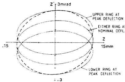
Fig. 8: Over deflected bunch centres at RF dipole exit, and "enclosing" ellipse (broken line).
