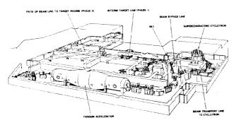
Fig. 1 The Chalk River Tandem Accelerator Superconducting Cyclotron system (TASCC).
