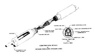
Fig.5 Typical construction of the cryogen transfer lines.
