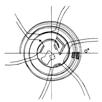
Fig 1. Electrode structure for the K500 first harmonic central region. Four orbits are shown corresponding to starting times  $\tau_0$ = 230,240,250, and 260 degrees. The peak electric field between source and puller is achieved at  $\tau_0$ =270. A slit is located on the 0° hill extension of the center plug allowing easy installation and removal. This slit removes all starting times which do not fall between 230 and 250 degrees.
