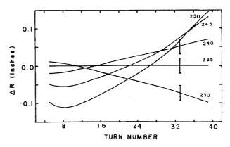
Fig 2. Radius difference  $r_i - r_0$  at  $\theta = 84^{\circ}$  vs turn number for a family of central rays. Ray 0 leaves the source at  $\tau_0 = 235^{\circ}$ , the others at the times labeled on the plot. At Turn 33 a bar of ±.02 inches in shown to give an idea of the radius variation expected from the r,pr distribution around the central ray.
