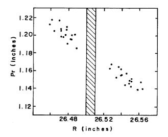
Fig 4. R is plotted versus Pr for turns 507 and 508 at  $\vartheta$  = 336 which corresponds to the entrance to the electrostatic deflector. Pr has been divided by the momentum unit mu<sub>0</sub> to express it in inches. The shaded area corresponds to a possible location for the deflector septum. This plot shows that single turn extraction of resulting beam should be possible. The energy spread of this group is less than 6 parts in 10<sup>4</sup>.
