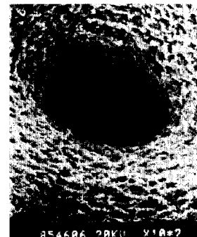
Fig. 2 Crater produced by sputtering of a series of electron beams on an iron target.
