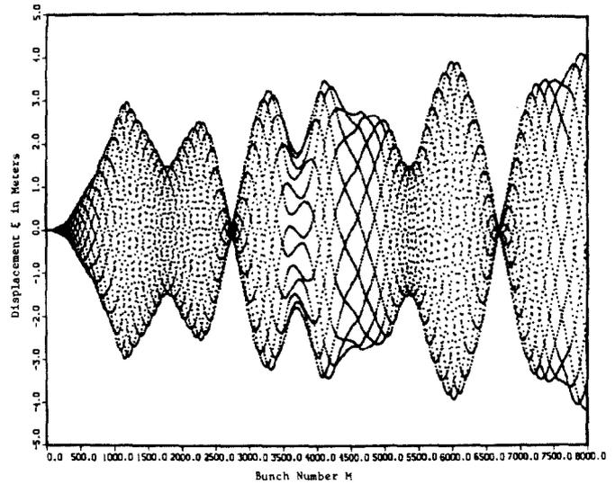
Fig. 2  $\xi(N, M)$  vs  $M$  for Cavity Number  $N = 30$  with Random Initial Displacement
