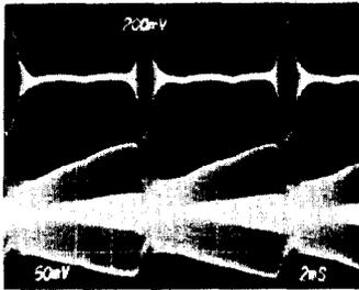
Fig. 4. Phase detector output (upper trace) shows growth of dipole oscillation coincides with dip in BME amplitude (lower trace).
