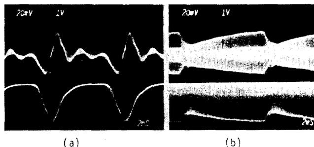
Fig. 1. Beam monitoring electrode signal (upper) and crossed-field photomultiplier output (lower), displayed at (a) 2 ns/div and (b) 2 ms/div, show slow fluctuation.
