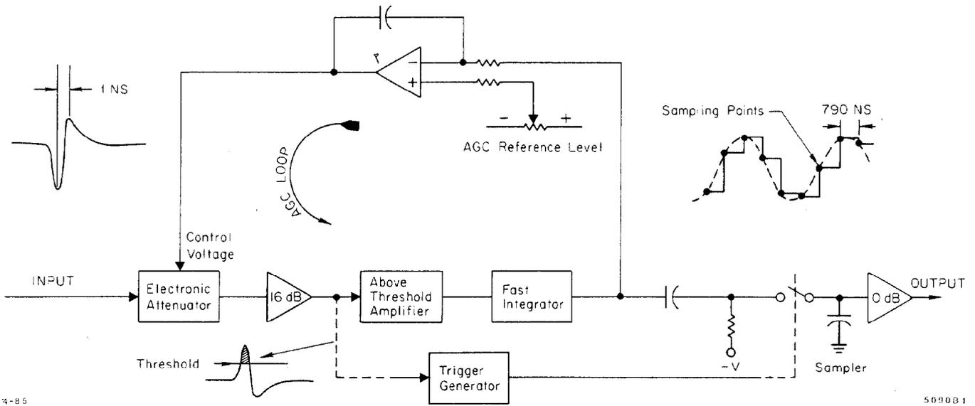
Fig. 1. Signal processor for the beam position monitor pulses.
