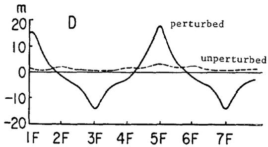
Fig. 4 Dispersion function in one superperiod when  $\gamma_T \approx 200$  in the harmonic scheme.
