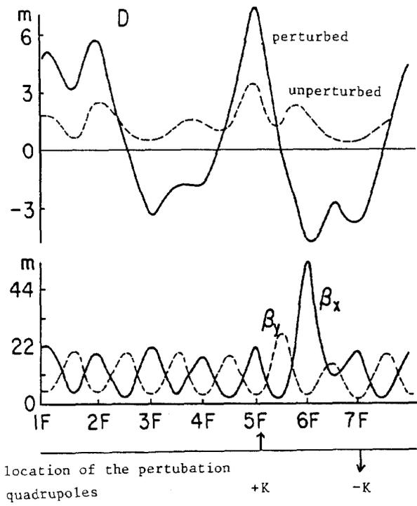
Fig. 3 Betatron oscillation parameters in one superperiod when  $\gamma_T$  is about 200 in the doublet scheme.
