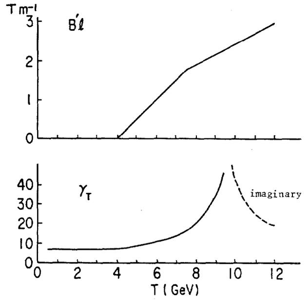
Fig. 5 Excitation curve of the doublet and the resultant  $\gamma_T$ .
