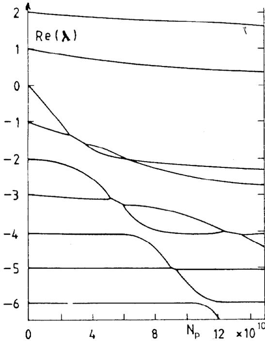
Fig.6 - Mode frequency versus current for the SPS at 315 GeV/c ( $\lambda = \omega - \omega_\beta / \omega_S$ ).
