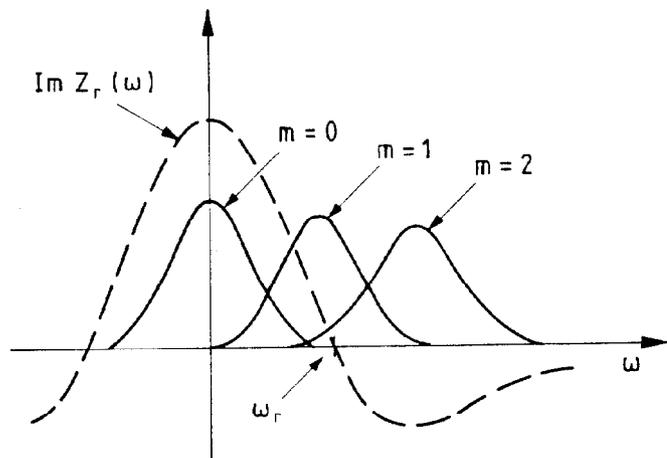
Fig.1 - Spectrum of the lowest modes with imaginary part of transverse broad-band impedance.
