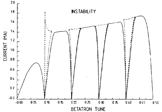
Fig. 3 - Threshold current as function of betatron tune from Vlasov equation with localized impedance.
