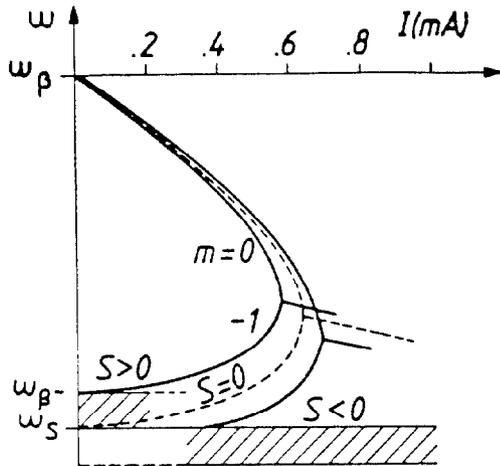
Fig.7 - Mode-coupling with synchrotron frequency spread.
