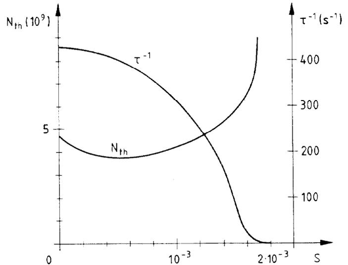
Fig.8 - Landau damping by betatron frequency spread.
