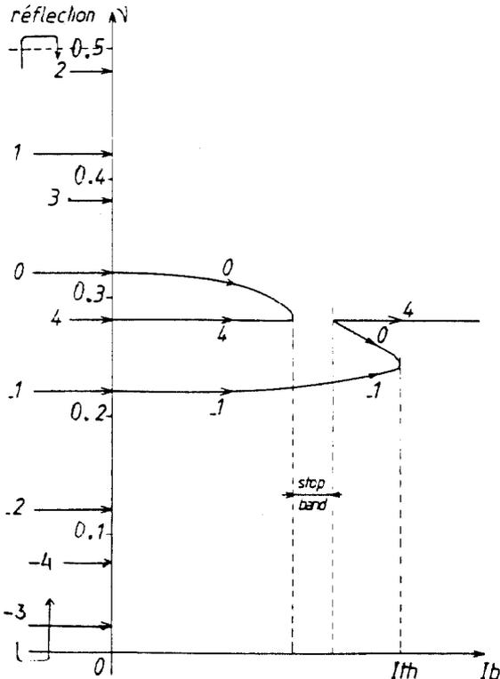
Fig. 2 - Mode frequencies versus bunch current from Vlasov equation with localized impedance.
