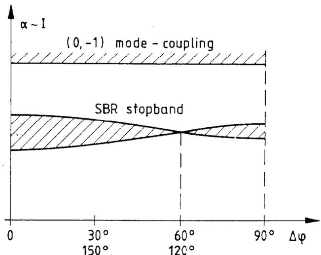
Fig.5 - Threshold versus phase-shift between 3 equally spaced cavities.
