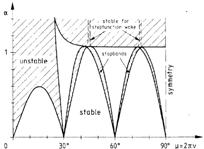
Fig.4 - Threshold kickstrength from two-particle model ( $\nu_s = 1/12$ ).
