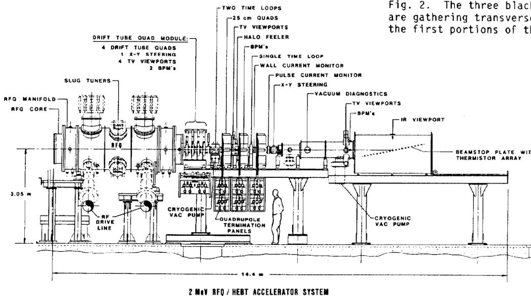
Fig. 1. HEBT sketch showing the relative placement of the diagnostic probes with respect to the other beamline components.
