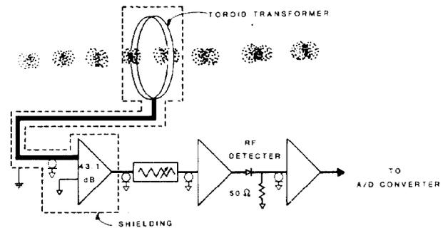
Fig. 5. The electronic detection circuitry for the toroid transformer.
