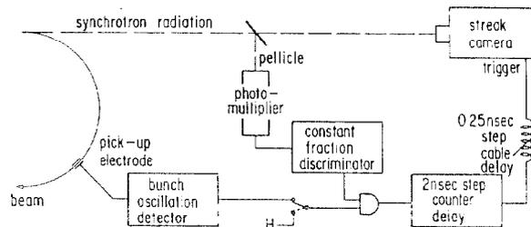
Fig. 1 Triggering of the streak camera.
