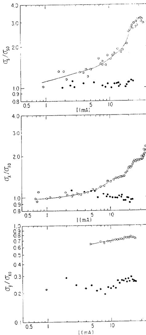
Fig2 Beam current dependence of bunch length, width and height.
