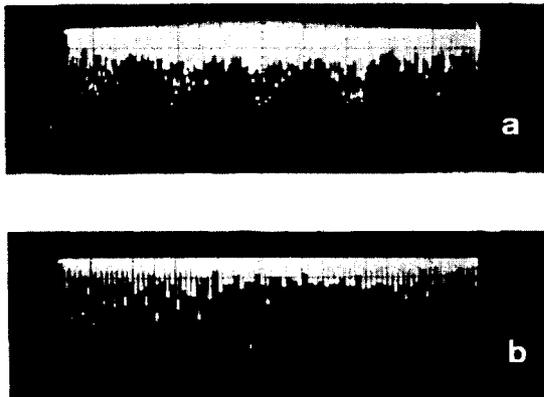
Fig. 6 Fine structure of the instability at its peak observed by waveforms of radiation intensity emitted from small central area of the transverse plane.
