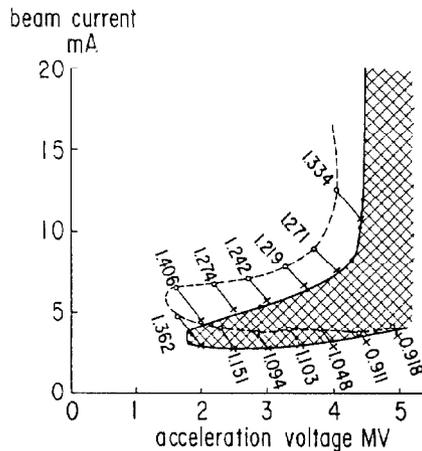
Fig. 5 Unstable region in the beam current-RF voltage plane with bunch length around it.
