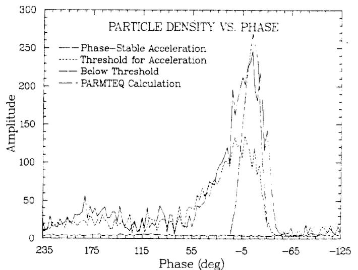
Fig. 5. Particle density versus the RFQ phase angle for RFQ power levels sufficient for phase-stable acceleration, at acceleration threshold, and below threshold. PARMTEQ calculations are indicated by the chain-dot curve.
