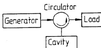
Fig. 4 A circulator to match the RF power generator
