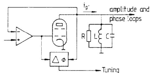
Fig. 6 RF feedback around the power amplifier
