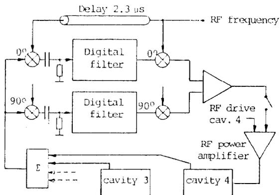
Fig. 7 Layout of the RF feedback system
