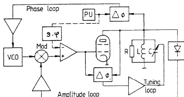
Fig. 5 Tuning, amplitude and phase loops
