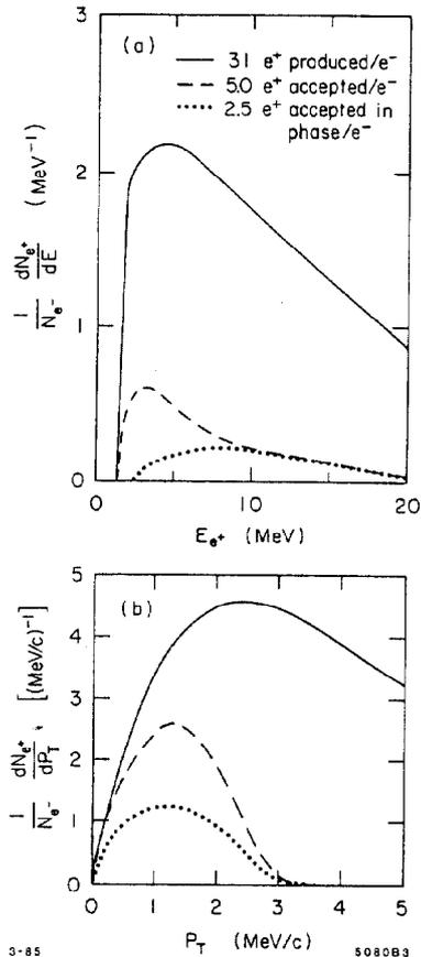
Fig. 6. Energy and transverse momentum of the positrons as they leave the target. Full curve shows all positrons produced, dashed curve gives the yield for positrons reaching the end of the accelerating system and the dotted curve shows those positrons in phase that would be accepted by the damping ring.
