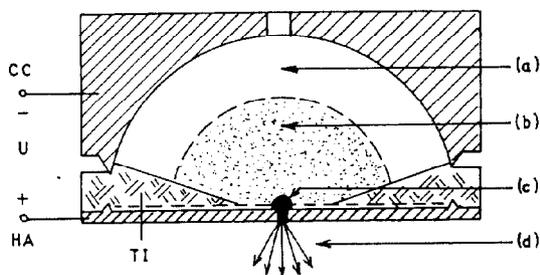
Fig.1. Schematic diagram of the hollow anode discharge: CC - concave cathode, HA - hollow anode, TI - teflon insulator; (a) - cathode dark space, (b) - negative glow, (c) - hollow anode glow, and (d) - outflow of the plasma.
