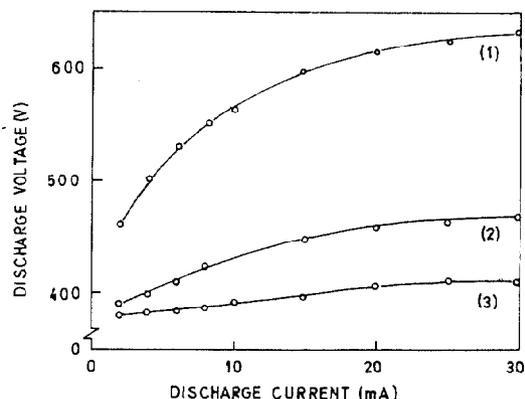
Fig. 3. Current-voltage characteristics of the ion source discharge for hydrogen pressure:  $p=1 \cdot 10^{-2}$  Torr - curve (1),  $p=3 \cdot 10^{-2}$  Torr - curve (2), and  $p=5 \cdot 10^{-2}$  Torr - curve (3).
