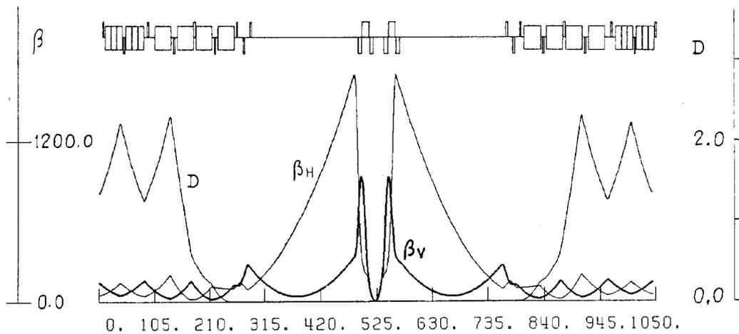
Fig. 4 Full insertion for LHC P-P-bar option, 10 quadrupoles per arm.
