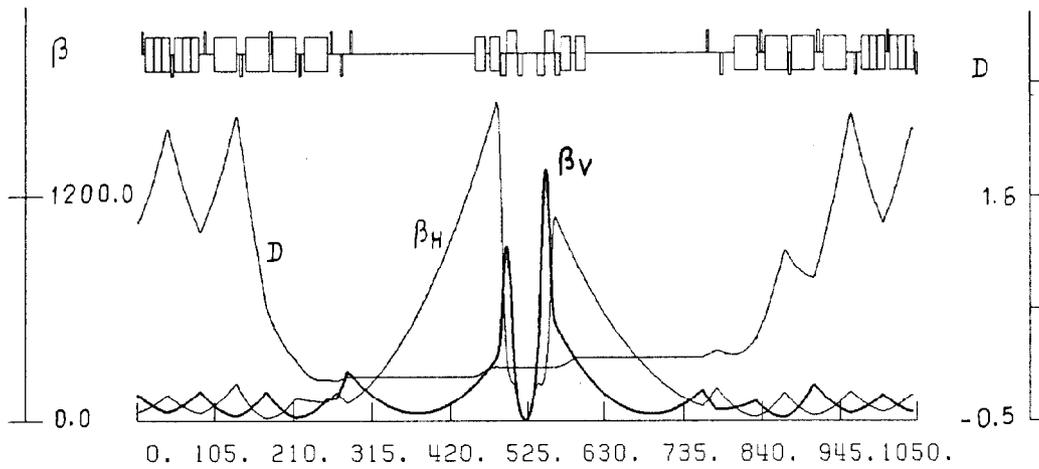
Fig. 3 Full insertion for LHC P-P option, 10 + 9 quadrupoles. Ring 1
