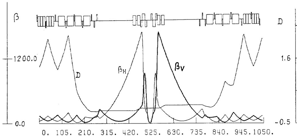
Fig. 2 Full insertion for LHC P-P option, 10 quadrupoles per arm, Ring 1
