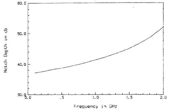
Figure 5. Calculated notch depth (ratio of peak to notch of T(f)) for a model CCF with notch dispersion and notch depth compensation.
