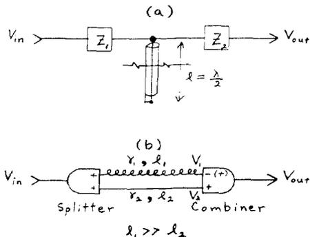
**Figure 1(a).** Schematic diagram for the commonly used shorted stub notch filter, (b) schematic diagram of the Basic Correlator Filter, with signal ( $V_1$ ) from a long length ( $l_1$ ) of low attenuation cable and signal ( $V_2$ ) from a short length ( $l_2$ ) of high attenuation cable combined in a  $180^\circ$  (-) or  $0^\circ$  (+) combiner.
