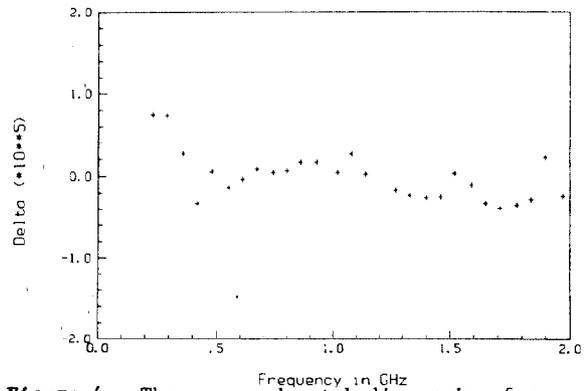
Figure 4. The measured notch dispersion for a prototype CCF with notch dispersion compensated for. Frequency spacing for the notch had  $f_o = 0.63$  MHz.
