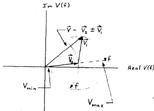
**Figure 2.** Phasor Diagram for the Basic Correlator Filter shown in Fig. 1(b). Also shown is the influence of the attenuation of the  $V_1$  signal on the notch ( $V_{min}$ ) and the influence of the phase dispersion of signal  $V_2$  on the phase at the notch.
