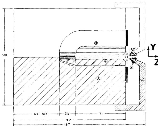
FIGURE 1. Side view of NBS-LANL RTM end magnet with the lower half shown in section. The magnet is 158 cm. long in the direction,  $x$ , perpendicular to this view. The  $y$ - $z$  section of this magnet is  $x$ -independent. All dimensions are in centimeters. Parts shown are: 1) main yoke, 2) main pole piece, 3) main coil, 4) active field-clamp coil, and 5) active field-clamp.
