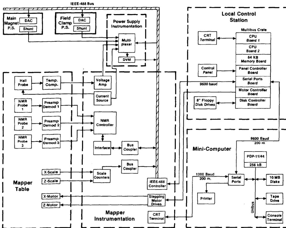
FIGURE 3. Block diagram of the data acquisition and control system.
