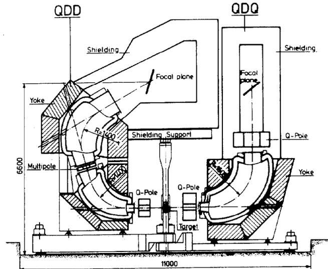
Fig. 4 The spectrometer pair installed at NIKHEF-K
