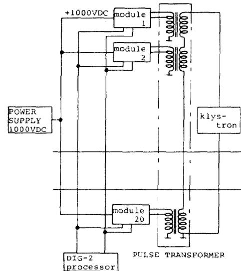
Fig. 2 Modulator block diagram
