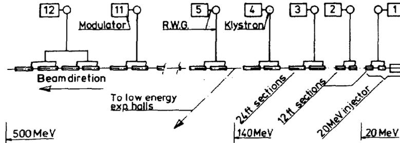
Fig. 1 Main components of the 500 MeV Linac
