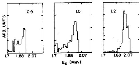
Fig. 4(b). Calculated output energy distributions for the RFQ at power levels of 0.9, 1.0, and 1.2 times the design power.
