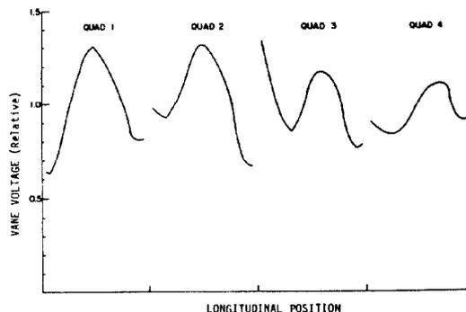
Fig. 1. Final intervane voltages as a function of longitudinal position. The distributions in each quadrant are normalized to 1.0.
