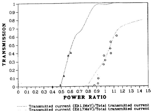
Fig. 5. Calculated transmissions through threshold Faraday cups for beam energies greater than  $\sim 1.1$  MeV compared with measured transmissions.
