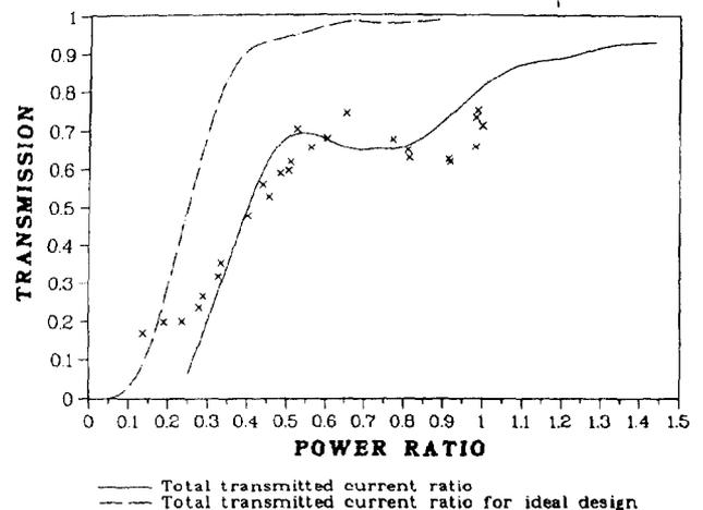
Fig. 3. Calculated and measured total transmission through the RFQ. The dashed curve represents the RFQ's expected transmission if field errors could have been eliminated.
