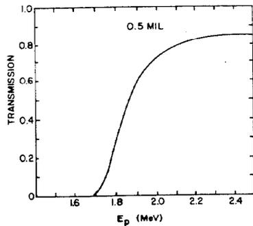
Fig. 4(a). Measured transmission curve for the 0.5-mil retarding foil of the threshold Faraday cup.
