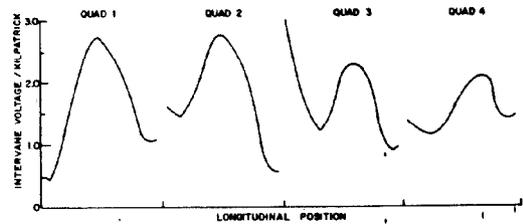
Fig. 6. A near repeat of Fig. 1, except that inter-vane voltages are calculated with 625.0-kW average power in the RFQ; resulting vane voltages have been referenced to the Kilpatrick spark criterion.
