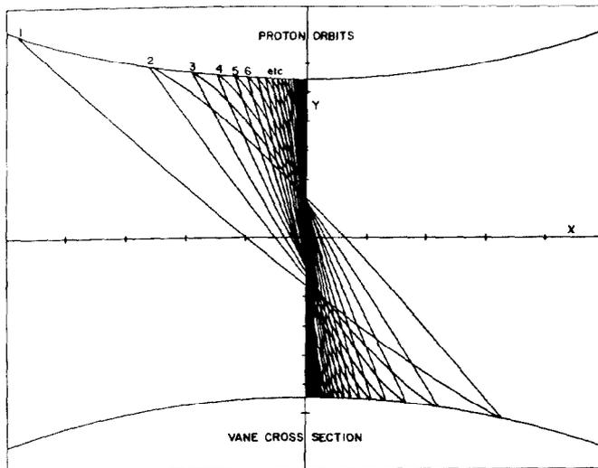
Fig. 2. Computer plot of the ion trajectories showing their stability and that they collapse rapidly to the vane center. This view looks along the RFQ axis.
