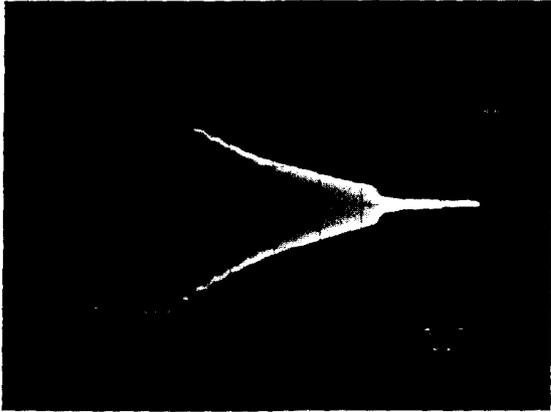
Fig. 3 - Tail of an RF pulse, evidencing multipacting levels. Vertical scale 100 KV/cm.-
