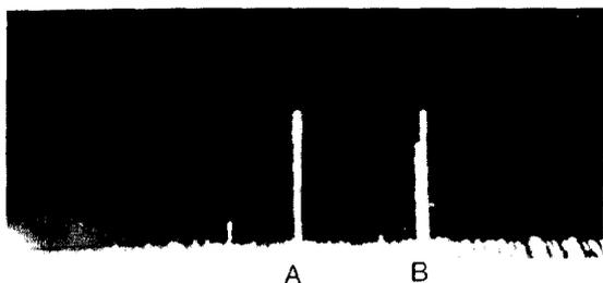
Figure 4. Spectrum analyser recording from an uncalibrated antenna monitoring the slotted waveguide at the klystron. Beam 600 MeV, stacking limiting at 80 mA due to an instability induced by turning off the octupole magnets and causing a large horizontal blow up.
