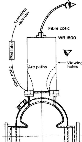
Figure 2. Method of observing and detecting waveguide arcs under no beam conditions.
