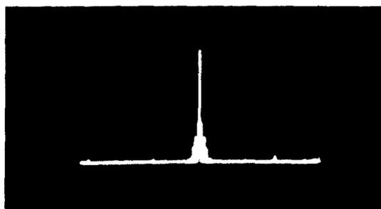
Figure 6. Spectrum analyser plot from storage ring diagnostic strip. 2 GeV 250 mA beam stored centre frequency 500 MHz. Scan 0-1000 MHz peak response 60 dB.
