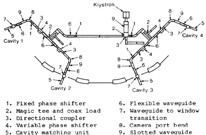
Figure 3. Showing composition and layout of SRS r.f. system as at 1st February 1983.
