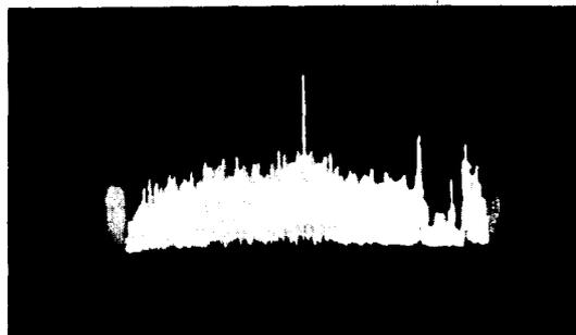
Figure 5. Spectrum analyser plot from the storage ring diagnostic strip with 2 GeV 220 mA beam stored centre frequency 500 MHz Scan 0-1000 MHz peak response 60 dB.
