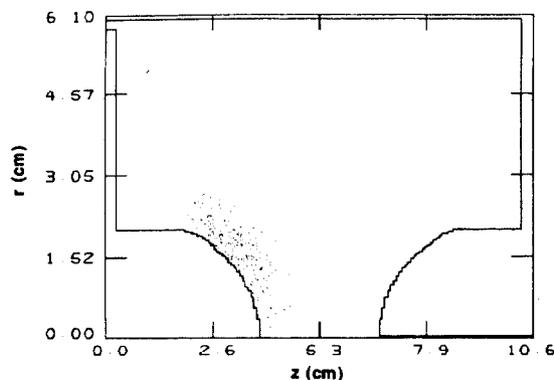
Fig. 3. Cavity simulation of the 1300 MHz resonator at Los Alamos (Ref. 21). Field emission (shown) and secondary emission (not shown) are important features of coding.
