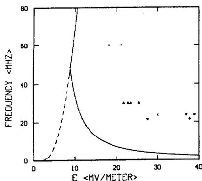
Fig. 1. Breakdown thresholds predicted by Kilpatrick (dashed curve) and by this study (solid curve) with experimental data points.
