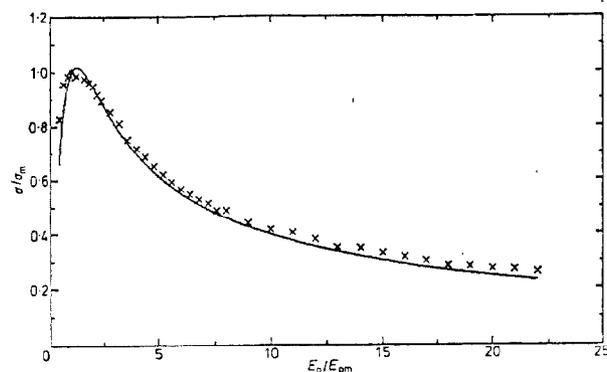
Fig. 2. Agarwal's universal yield curve for secondary emission as a function of primary energy with corresponding data points (Ref. 20).
