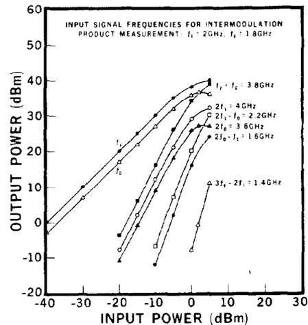
Fig. 4 Typical performance characteristics of the 2-4 GHz traveling-wave tube amplifier.
