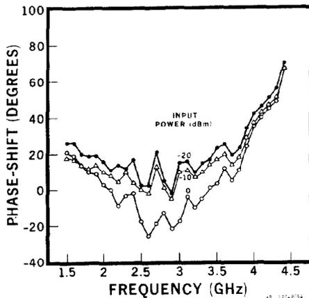
Fig. 2 Amplifier phase-shift as a function of frequency with the input power level as parameter.
