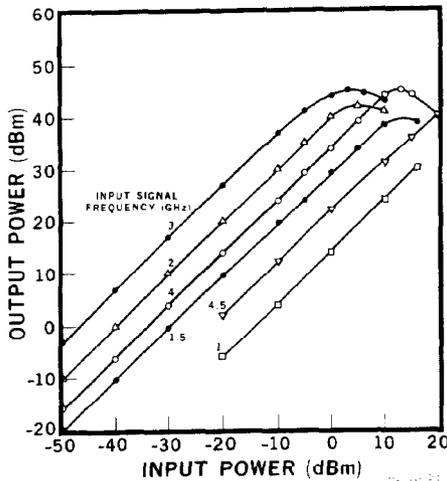
Fig. 1 Output power as a function of the input power level with the input signal frequency as parameter.
