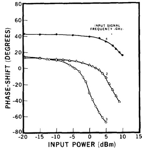
Fig. 3 Amplifier phase-shift characteristics as a function of the input power level with input signal frequency as parameter.
