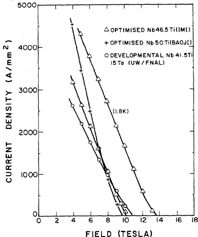
Fig. 1.  $J_c$  ( $10^{-14} \Omega m$ ) results on some recent high  $J_c$  conductors. Values are at 4.2 K except where noted.
