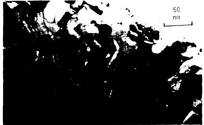
Fig. 3.  $\alpha$ -Ti precipitates in a transverse section of an optimized Nb 50 wt% Ti composite ( $J_c$  5 T, 4.2 K = 2610 A/mm<sup>2</sup>). Courtesy of Anne West.
