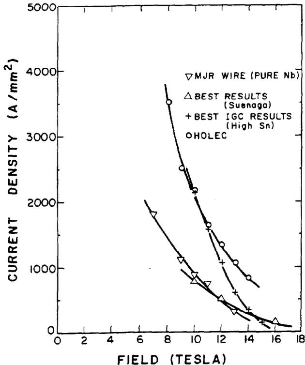
Fig. 2.  $J_c$  results on some recent high  $J_c$  Nb<sub>3</sub>Sn conductors.  $J_c$  values are at various criteria (see text). Data is included from references 22, 23, 32, 33. The lower two curves are for bronze route conductors, the upper for high Sn process material.
