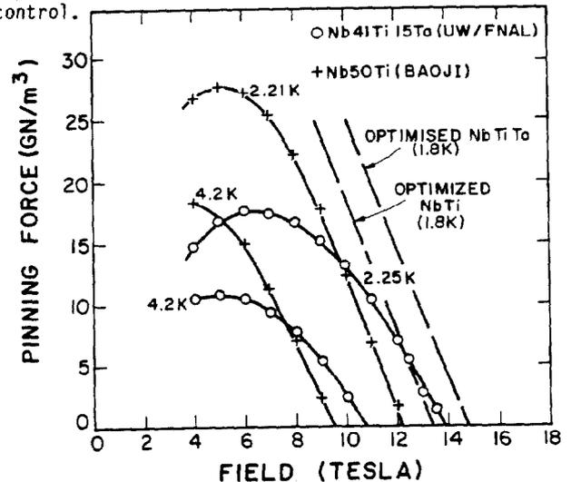
Fig. 5. Pinning force ( $J_c \times B$ ) curves for Nb-Ti and Nb-Ti-Ta conductors (see also Fig. 2). The dashed lines are scaled from the 2.21 K high field slope of the Baoji conductor, using the maximum  $H_{c2}$  values expected from binary and ternary alloys at 1.8 K (see text).
