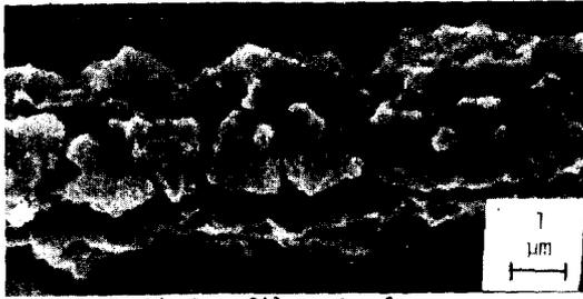
Fig. 4. Reacted  $\text{Nb}_3\text{Sn}$  filament from a composite having initially strong pre-reaction. The uneven cross-section is very evident. Courtesy of David Smathers.
