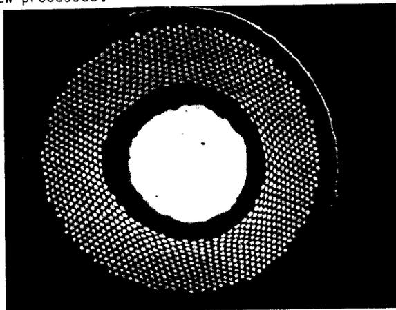
Fig. 7 Tin-core conductor made by IGC. The central core is Sn, the outer section containing Nb filaments embedded in copper. (Courtesy of R. E. Schwall.)
