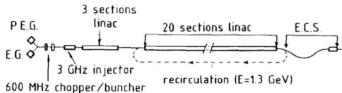
Fig. 3 - Layout of the new linac (100  $\mu\text{A}$ , 1.3 GeV without recirculation, 2 GeV with recirculation). P.E.G.: polarized electron gun; E.C.S.: energy compression system.
