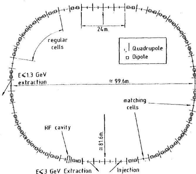
Fig. 5 - The stretcher ring (circumference : 300 m. ; magnetic radius  $\rho = 15 \text{ m.}$ ).
