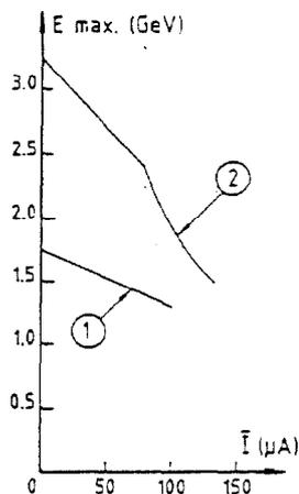
Fig. 4 - Characteristics of the modified linac; (1) without recirculation; (2) with recirculation.
