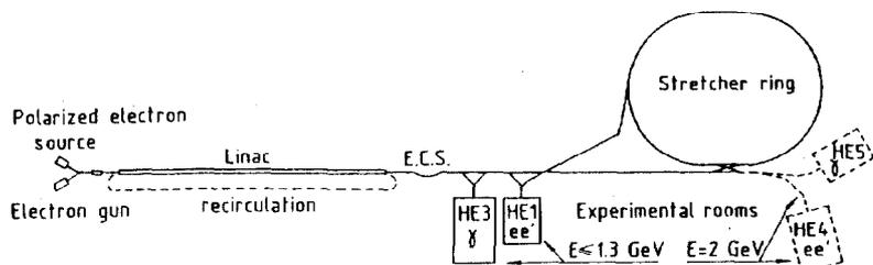
Fig. 1 - Layout of the new facility designed at ALS Saclay. 1st stage : 1.3 GeV, 100 % d.c. 2nd stage : 2 to 3 GeV (dashed lines).
