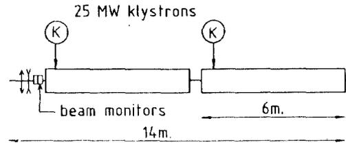
Fig. 2 - Linac elementary cell; energy gain ( $i \approx 0$ ) 150 MeV, ( $\bar{i} = 100 \mu\text{A}$ ) 110 MeV. Klystron duty cycle  $\geq 10^{-3}$  at 25 MW.
