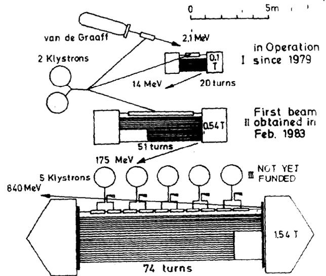
Fig. 1: Scaled scheme of the MAMI project
