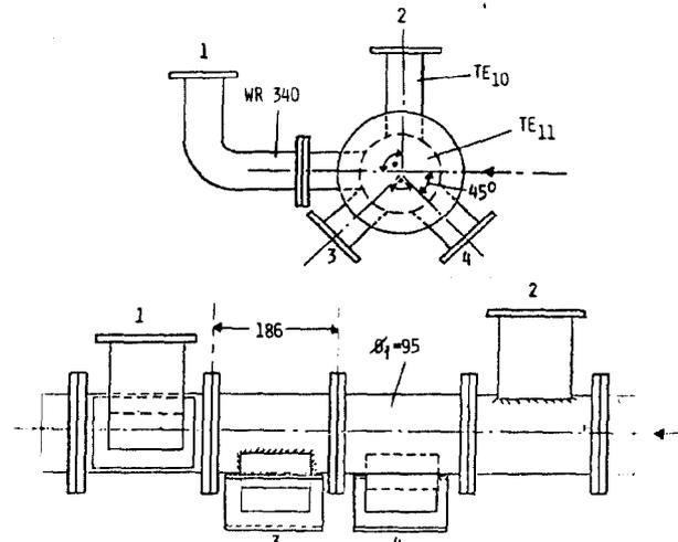
Fig. 7: A circular magic T power combiner/divider
