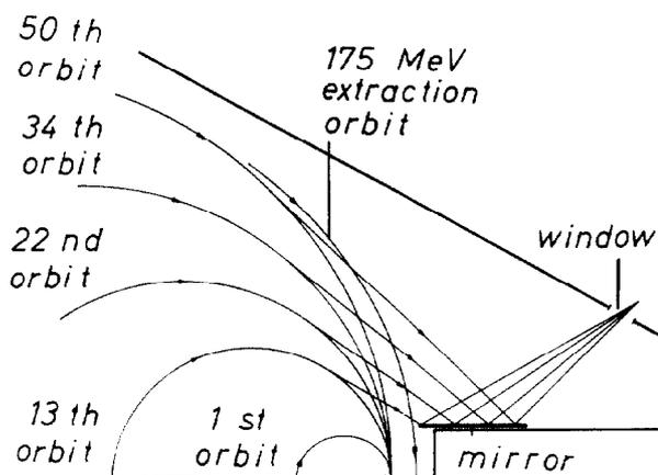
Fig. 8: Layout of the synchrotron light monitor
