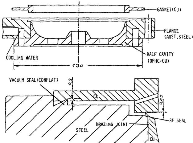
Fig. 5: The vacuum-rf-seal for the sections of stage II
