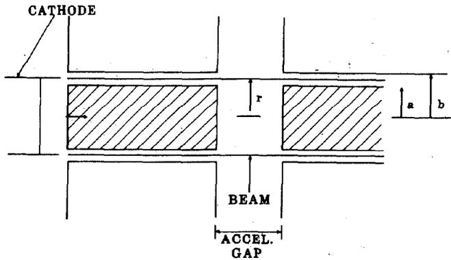
Figure 5. Cross-sectional view of a coaxial drift tube transport system.
