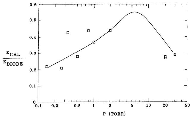
Figure 2. Ratio of apertured transported energy ( $R < 2.5$  cm) to injected diode energy vs. pressure for a cathode  $B_z = 3.7$  kG.
