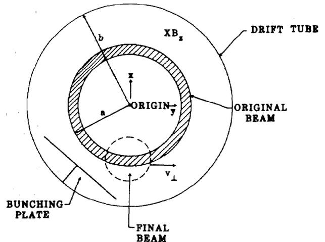
Figure 6. Idealized cross-sectional geometry of the  $P_\theta$  elimination technique.
