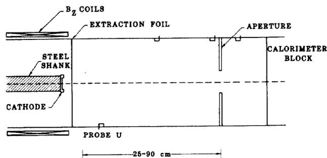
Figure 1. Gas propagation experimental configuration.
