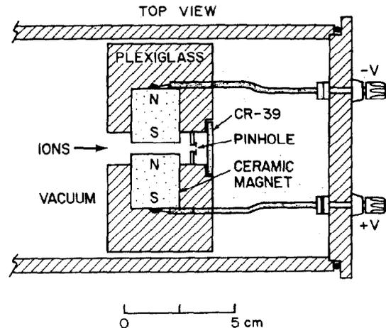
FIG. 3. Cross sectional view of Thomson spectrometer.
