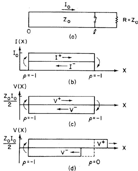
FIG. 1(a). Transmission line initially shorted at both ends and current charged with  $I_0$ , (b) Superposition of two waves  $I^+$  and  $I^-$ , (c)  $V^+$  and  $V^-$ . (d) When the switch opens,  $V^+ = Z_0 I_0/2$  and  $I^+ = I_0/2$  proceeds towards the matched load.
