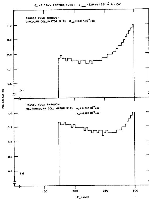
Fig. 9 Tagged- $\gamma$ -polarization for 2 collimator shapes.
