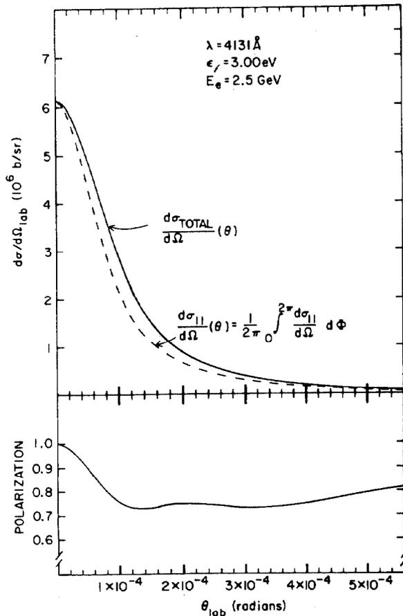
Fig. 8 Angular dependence of the  $\gamma$ -ray polarization.
