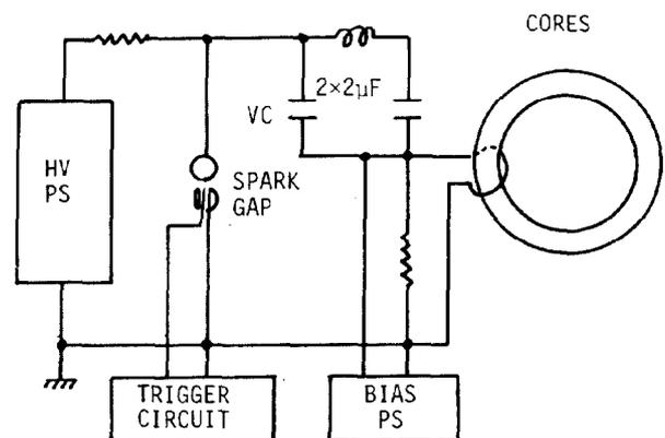
Fig.2 Electrical schematic of the driving circuit.
