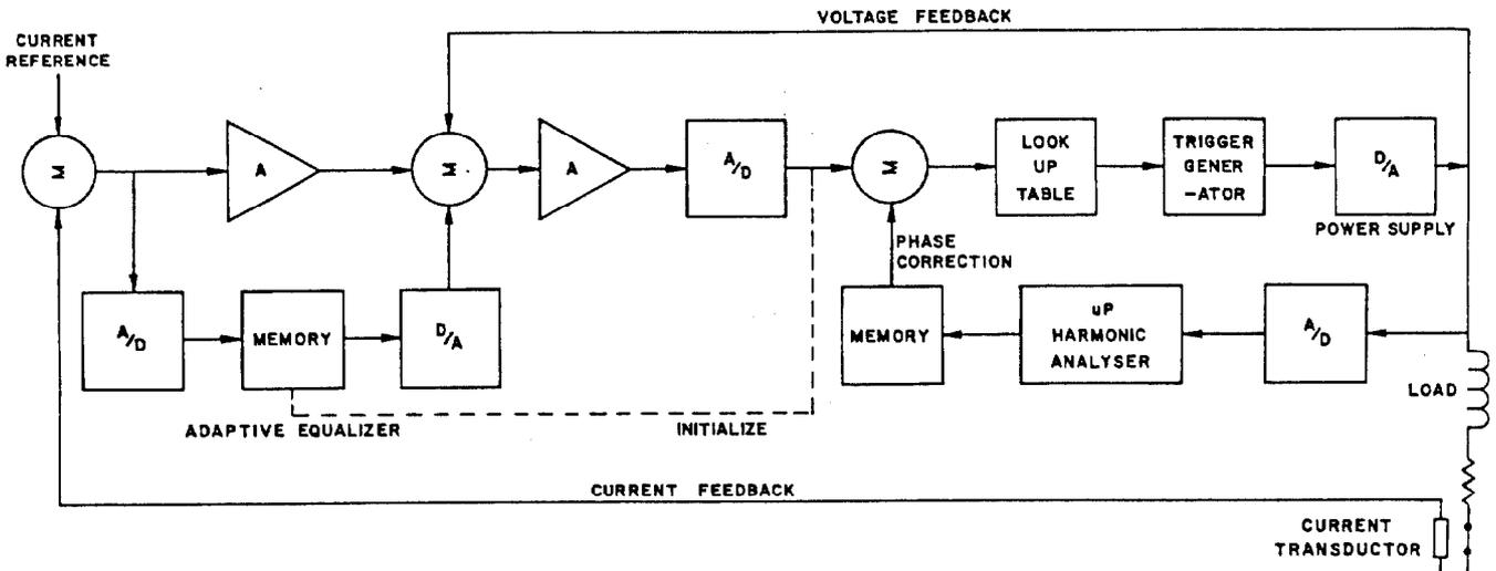
Fig. 3. Functional Block Diagram of the VUV Dipole Power Supply.
