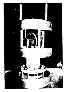
Fig. 1. The pressurized spark-gap assembly.
