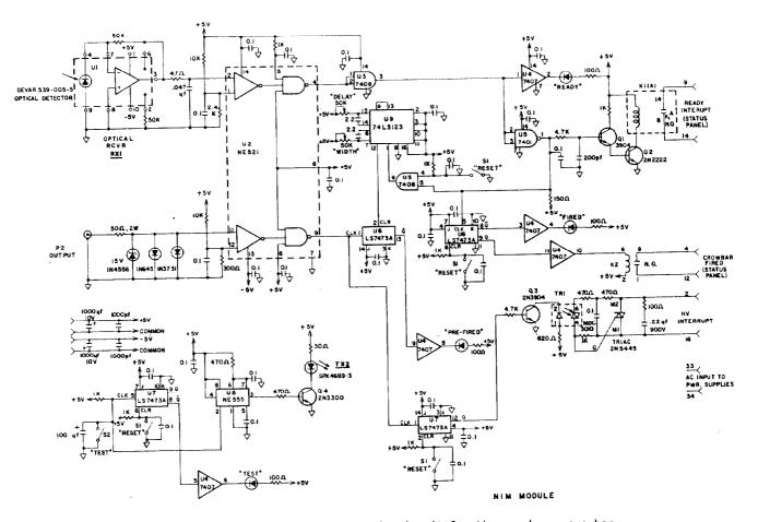
Fig. 3. Schematic of test and diagnostic circuit for the spark-gap crowbar.
