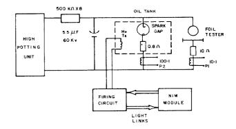
Fig. 4. Schematic of spark-gap crowbar test.
