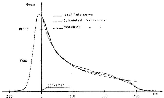
Fig. 4 Tapered field of the matching device
