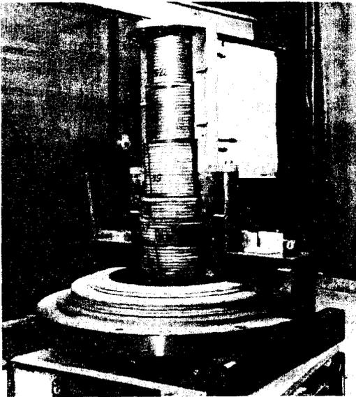
Fig. 5 Solenoid being assembled
