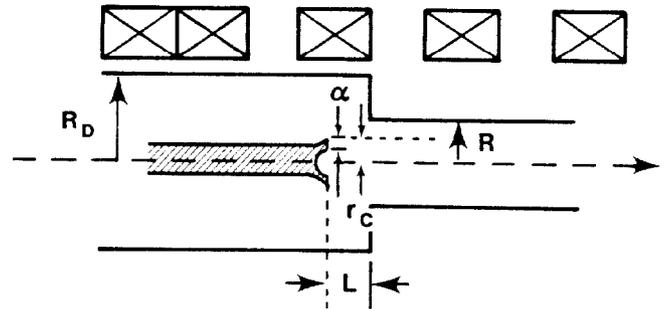
Fig. 4. Schematic design of the IBEX foilless diode structure.
