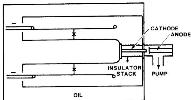
Fig. 2. Schematic diagram of the cylindrical isolated Blumlein PFL showing the symmetric charge line feeds, the oil switch location, the high voltage vacuum insulator stack, and a planar diode.
