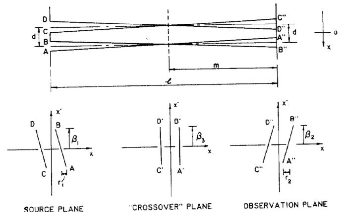
Fig. 2 Geometry and phase space plots of two beamlet system.
