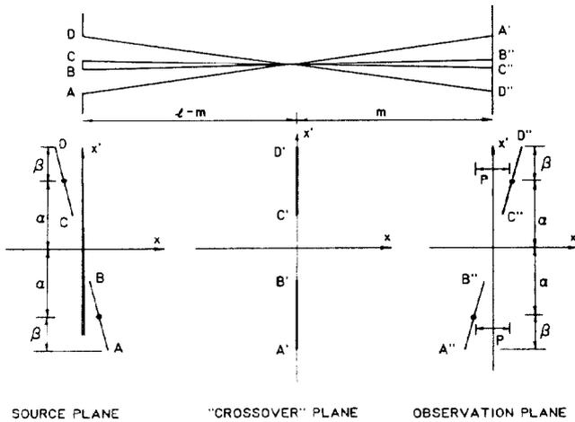
Fig. 3 Geometry and phase space plots of stacked beamlets.
