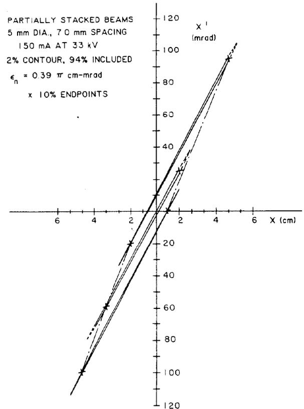
Fig. 4 Measured phase space plot of partially stacked beams.
