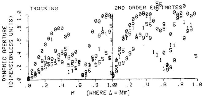
Fig. 4 Dynamic aperture over a range of  $\Delta$ 's for several insertions phases,  $\phi = \#(\pi/10)$ .
