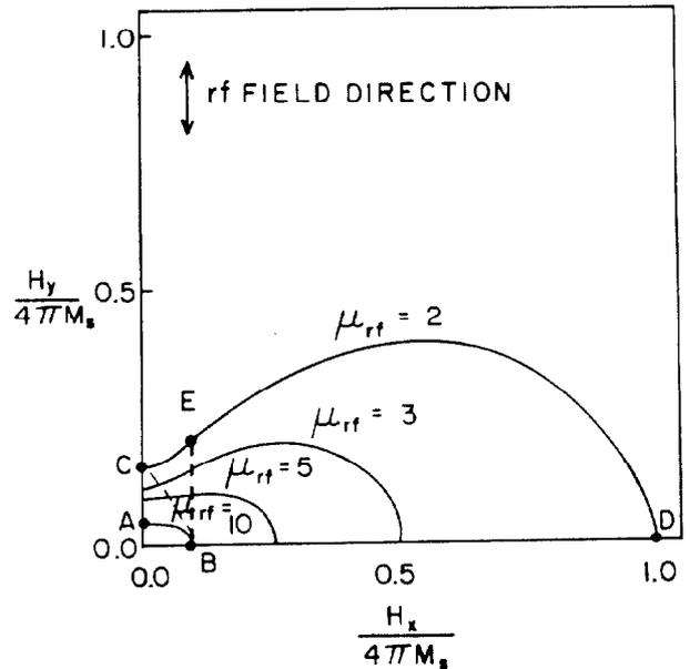
Fig. 3. A contour plot of the differential permeability in the y direction as a function of  $H_x$  and  $H_y$ , the magnetic bias field components. Values were calculated from Eqn. 8 with an initial permeability ( $\mu$ ) equal to 20. It is seen that tuning from B to C along the dashed path requires much smaller bias fields than tuning from B to D. Another alternative would be to apply a dc bias field in the x direction and a variable bias in the y direction, tuning from B to E.
