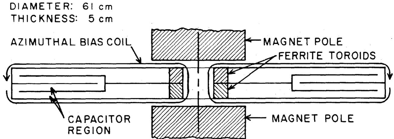
Fig. 4. Cross section of a cavity for testing ferrite. The thin, annular cavity is bisected by a conducting disc on the median plane. The disc carries the rf current from the capacitor region to the center of the cavity, passing between the two ferrite toroids.
