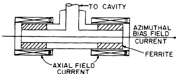
Fig. 1. A sketch of a ferrite tuner, consisting of a coaxial line which tees into two coaxial shorted stubs containing annular ferrite cylinders. The rf magnetic fields and the parallel bias field are in the azimuthal direction in the ferrite. An axial bias field which would be perpendicular to the rf magnetic field could be produced by the solenoidal coils.
