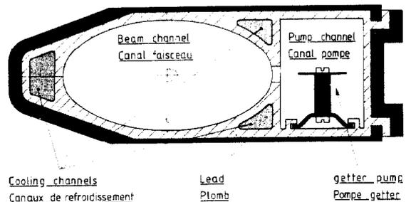
Fig. 6 : Cross-section of the dipole vacuum chamber
