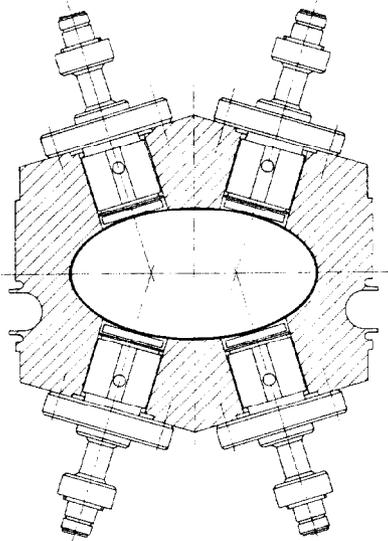
Fig. 7 : Cross-section of the pick-ups
