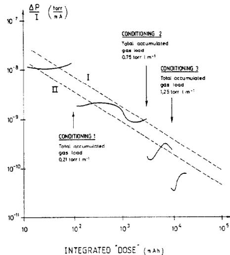
Fig. 5 : A typical pump-down curve
