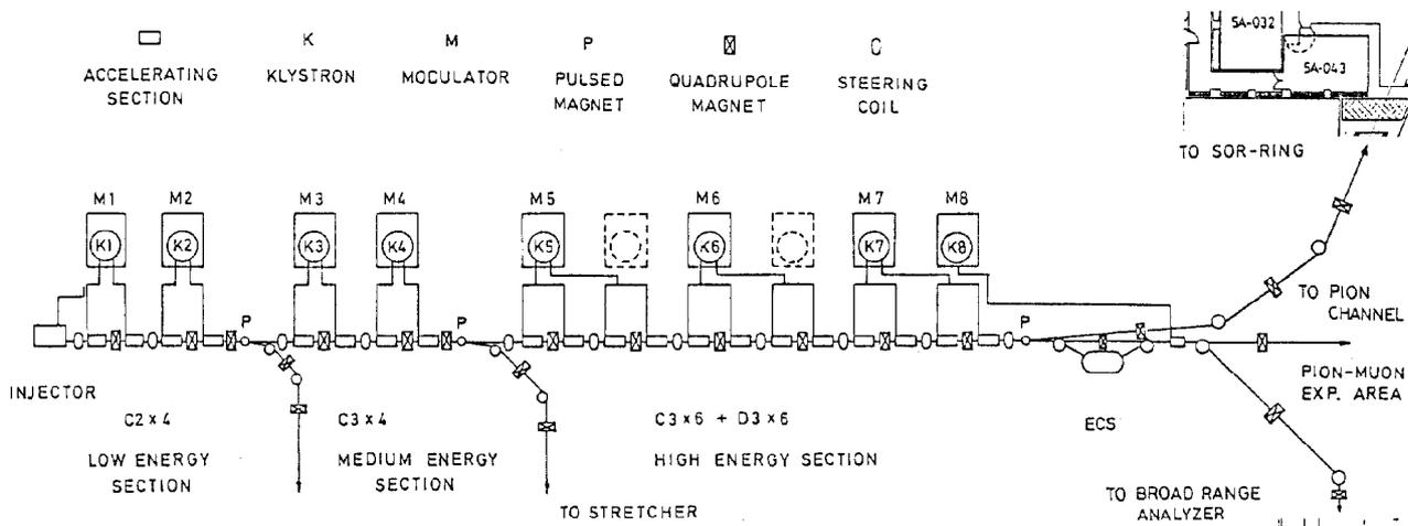
FIG. 4 Schematic Layout of the Beam Centerline, Klystrons, Modulators, and Beam Transport Systems.
