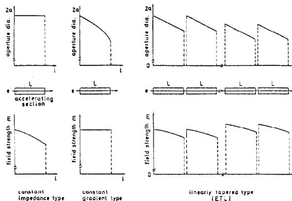
FIG. 2 Features of the Linearly Tapered Iris Type Accelerating Sections and Their Configuration.
