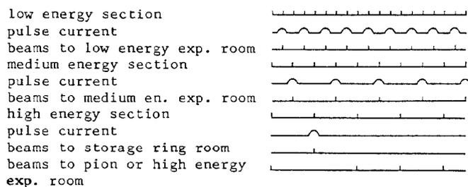
FIG. 6 Beam Sharing at Each Energy Section
