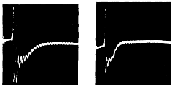
Fig. 1 (one feed) Fig. 2 (two feed) Transient phase shift during build up time. vertical: 18^\circ/\text{div} . horizontal: 20 \mu\text{sec}/\text{div} .
