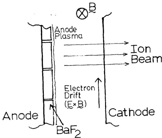
Fig. 1 Cross sectional view of diode gap.
