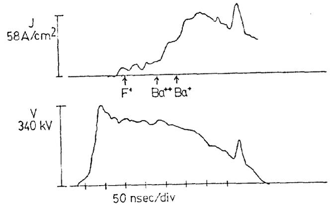
Fig. 2 Diode voltage and time-of-flight ion current for used anode.
