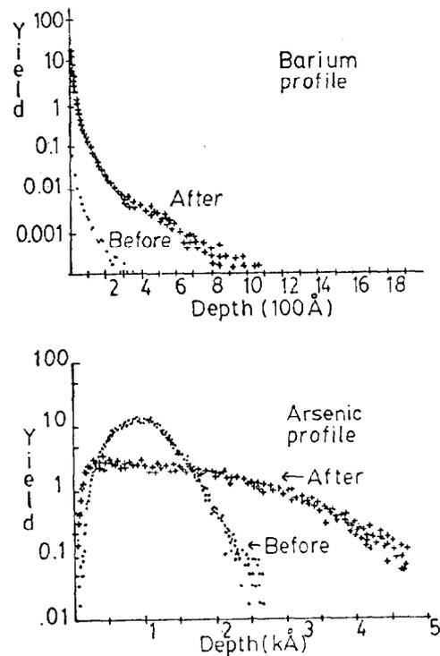
Fig. 4 SIMS analysis of arsenic implanted silicon crystal before and after treatment with barium beam.
