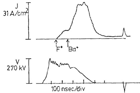
Fig. 3 Diode voltage and time-of-flight ion current for new anode.
