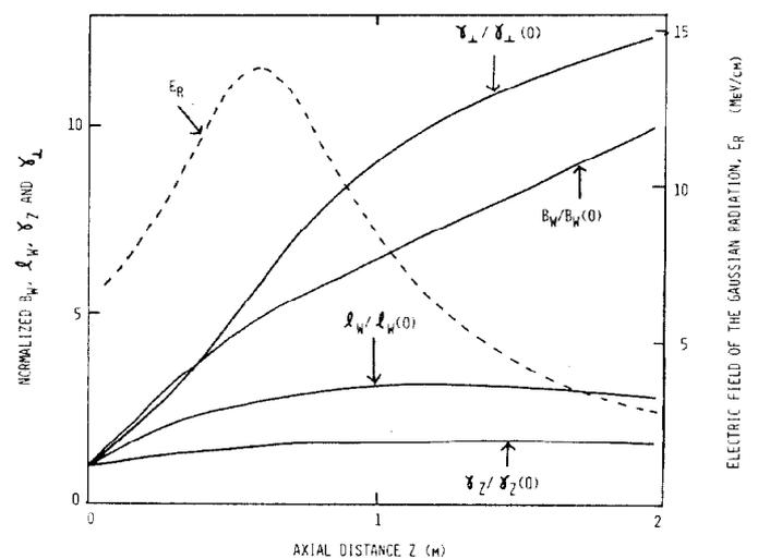
Fig. 4. Plots of the fundamental Gaussian free space diffracted radiation beam, and normalized  $B_w$ ,  $l_w$ ,  $\gamma_w$  and  $\gamma_{\perp}$  as a function of axial distance  $z$ .
