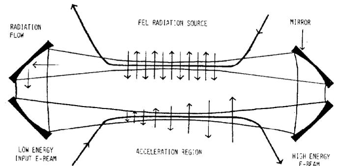
Fig. 3. Schematic diagram of the acceleration process utilizing the radiation field obtained from an FEL.
