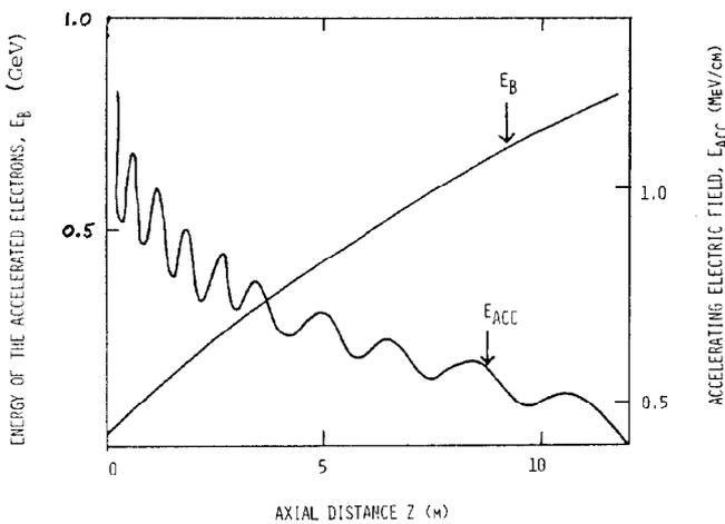
Fig. 2. Plots of the effective accelerating electric field,  $E_{acc}$ , and the energy of the accelerated electrons,  $E_b$ , as a function of axial distance  $z$ .
