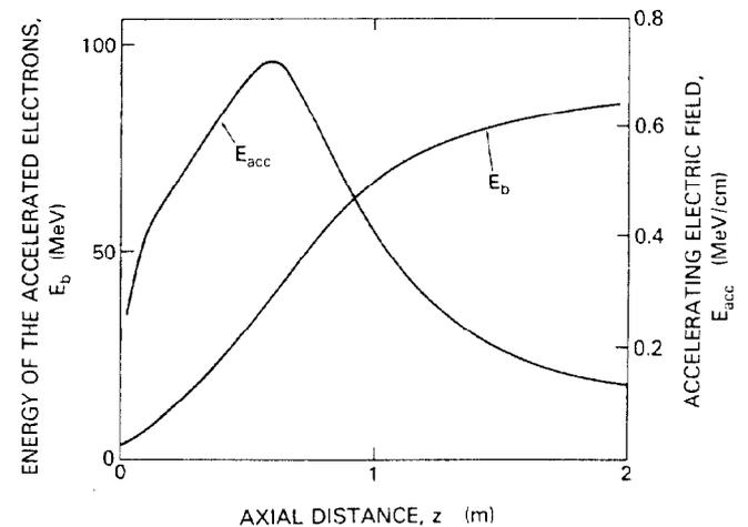
Fig. 5. Plots of the effective accelerating electric field,  $E_{acc}$ , and the energy of the accelerated electrons,  $E_b$ , as a function of axial distance  $z$ .
