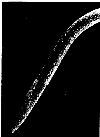
Fig. 4. Slip plane between grain boundary.
